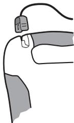
The *DDU-100* AED is designed to be stored with the defibrillation pad connector attached to the unit, while the pads themselves remain sealed in their package. This reduces the time needed to setup and start treatment in an emergency. The Defibtech AED should be stored with the pad connector plugged into the unit. However, if pads were damaged or not properly connected, you may need to substitute a new set of pads during an emergency. The pad connector is on the corner of the AED.
